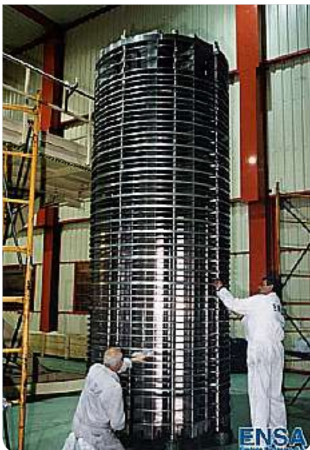
Figure 1. ENSA-DPT container internals: cooling discs and frame
