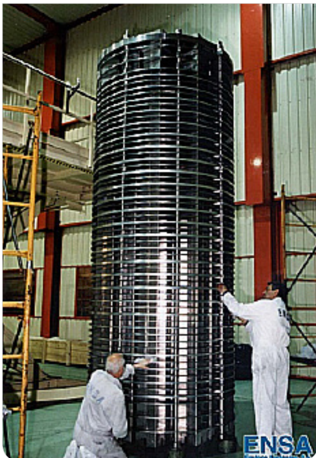
Figure 1. ENSA-DPT container internals: cooling discs and frame
